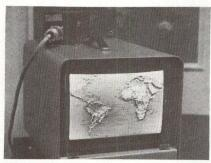
Capable of capturing an image with 64 levels of grey scale and 512 x 512 pixel resolution in 0.033 s and storing
