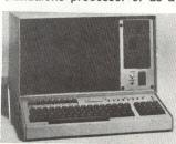
system. Features include a 15" (38-cm) high-resolution monitor; u/Ic ASCII keyboard with eight user-designated special function keys and 16-key numeric cluster pad; and Shugart SA-400 minifloppy disc drive. The 12-slot mainframe contains a CPU board with 8080 processor and a
