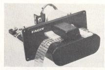
For use with microcomputer systems and terminals, 4031 is a bidirectional reader, with speed of 0 to 120 char/s asynchronous. With up to 60% transmissivity, it can be converted for 5-, 6-, 7-, and 8-channel tapes. Control electronics are on one board containing read head with light source connector for motor and connectors for I/O signals to the reader. It fits into a 2-module, 19" (48-cm) rack panel. Facit-Addo, Inc, 66 Field Point Rd, Greenwich, CT 06830.
