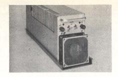
supplies input for dc-dc converter (outputs 2 and 3). Reduction in UPS section by 25% to outputs 2 and 3 provides 268 W or 48 Vdc at 6 A. Trio Labs, Inc. 80 Dupont St, Plainview, NY 11803.
