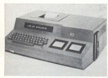
DE68DT microcomputer is self-contained with integral tape drives, alphanumeric/numeric display and printer, keyboard, miniature floppy disc, and RS-232-C. Both desktop and compact portable models are available from Digital Electronics
