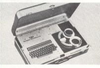
A portable, interactive terminal capable of interfacing to any mini/microcomputer via an RS-232 or current-loop port at selectable data transmission speeds from 110 to 9600 baud, CO-4420 consists of 1M-byte direct access tape drive, full ASCII keyboard, 40-char plasma display, RS-232 port, and microprocessor controller. Together in a compact case, they weigh only 23 lb (10.5 kg). LINCtape drive provides reliable mass storage. Computer Operations, Inc, 9700-B Palmer Hwy, Lanham, MD 20801.
